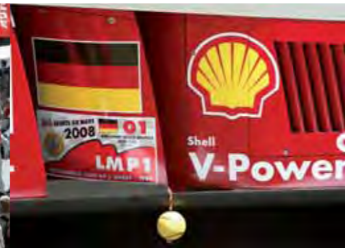
These little balls linked to carbon plates are there to remind the mechanics to remove the protection placed in front of the radiators.
